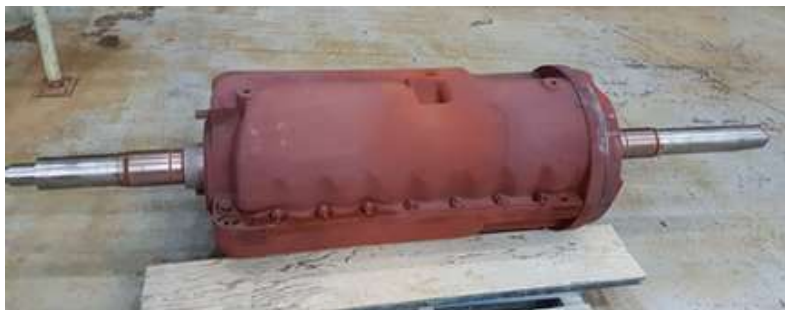
Figure 2: Refurbished Volute Impeller Cartridge.
